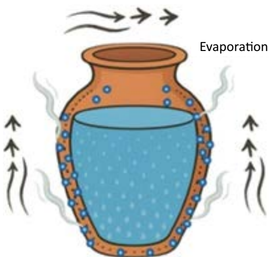
FIGURE 50 Cooling mechanism in earthen pots 93
