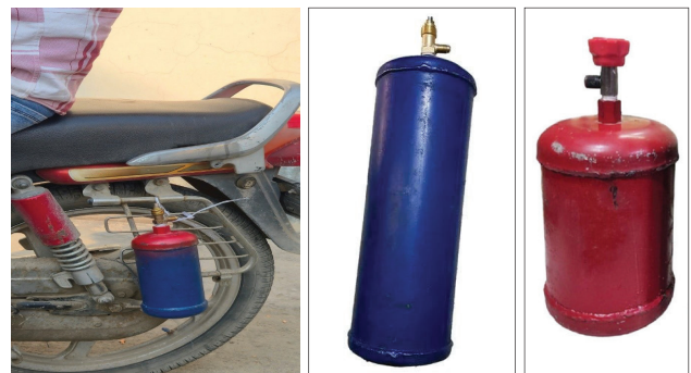
Figure 1 Unsafe cylinder transport on a two-wheeler (left) and examples of locally used refrigerant cylinders (right), highlighting risks associated with improper handling
