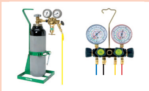
Figure 8.3 Two Stage Pressure Regulator
