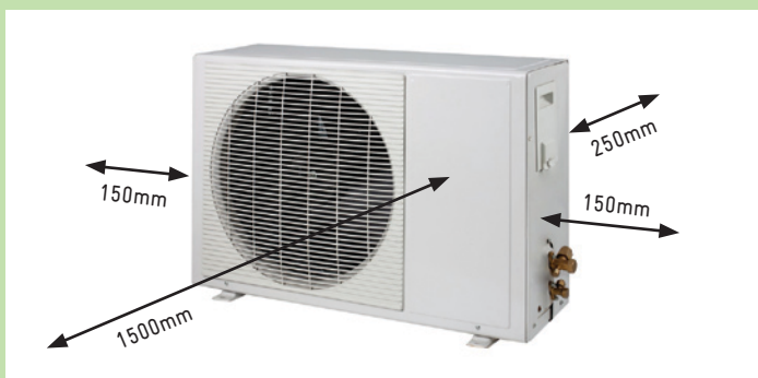
Figure 6.5 Proper Location for Outdoor Unit (ODU)
