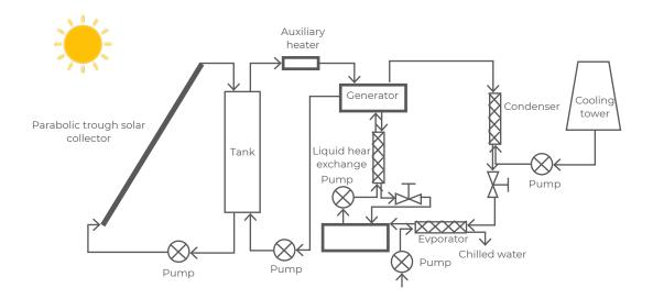
Figure 16: VAM supported by solar thermal collector Image Source: Renewable Energy and Energy Efficiency Group, The University of Melbourne
