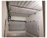
Figure 17: Reefer truck with eutectic plates
