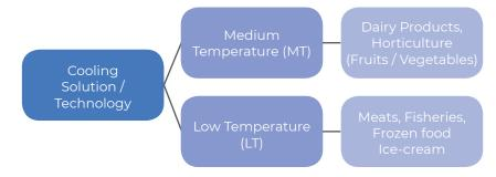
Figure 7: Cooling technology classification basis temperature
