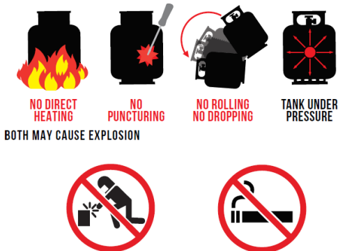
Figure 6: Prohibited activities in cylinder storage area
