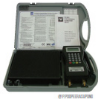
Figure 9: Refrigerant Charging Equipment
