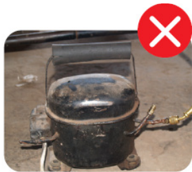
Figure 8: Compressors must not be used for vacuuming
