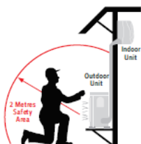
Figure 5: Temporary flammable zone
