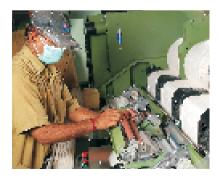
Picture 5: Cleaning of rollers in comber
