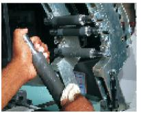
Picture 6: Cleaning of rollers in Drawframes
