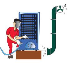
LEVs capture contaminants before they disperse into the air of the workplace. Such systems consist of a hood, a duct and an air cleaner. LEVs cannot be bought off the shelf and they have to be sized by experts to meet the specific requirements.
