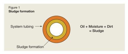
This includes petrol, anti moist, and air from leak testing, self evacuation and filling. Contaminants also enter when the circuitry is kept open for a long time during servicing. Over time, contaminants present in the system get circulated and, under high temperature and pressure, turn gradually to sludge.
