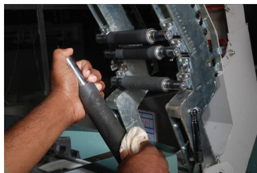
Figure 2: Cleaning of roller (dismantled)
