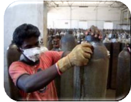
Figure 3: Cleaning of cylinder surface
