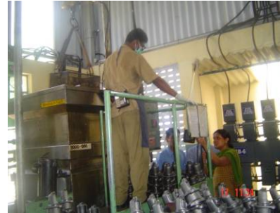
Figure 4: Cleaning of components by vapour degreasing method
