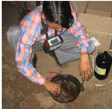
Figure 1: Cleaning of component by immersion
