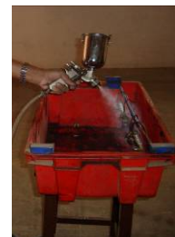
Figure 2: Cleaning of components by spraying method
