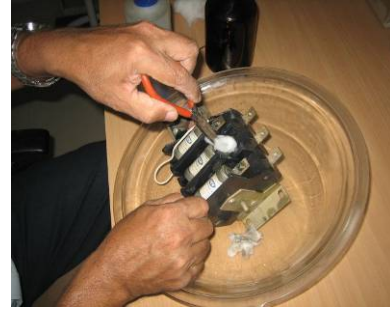
Figure 3: Cleaning of electrical contact by wiping method using nose plier
