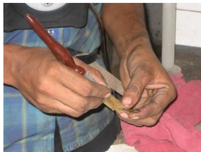
Figure 1: Cleaning of electrical contact by brushing method
