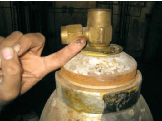
Picture 1: Oil and grease contaminants
