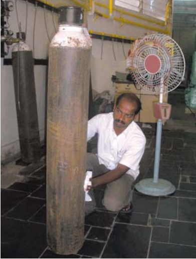
Picture 6: Downwind working position – reduces inhalation exposure levels
