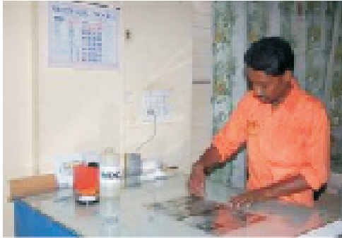
Picture 1: Mounting the film with cello tapes
