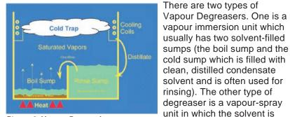
Picture 8: Vapour Degreasing
