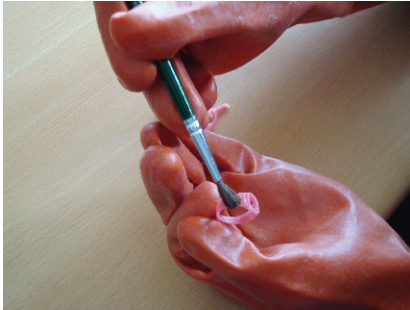
Picture 4: Finishing of wax pattern
