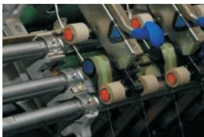
Picture 11: Rubber cots/ aprons in spinning
