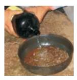
Scrap metal forms a major source of raw materials to foundries. Scrap collected from different sources will contain a lot of contaminants. To decide the actual weight of the metallic part in the scrap, a sample quantity is rinsed with solvents like CTC and then dried through heating. The difference in weight of the sample before and after rinsing determines the quantum
