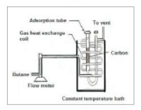
Picture 4: Apparatus for Butane activity test
